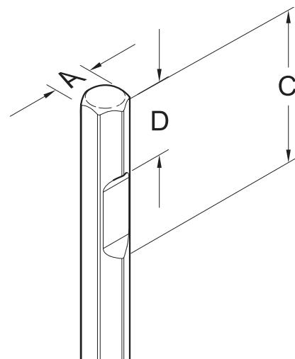
Use the gauge that corresponds to the insertion tool's shank dimension. See section "Technical data" for correct tool shank dimensions.
