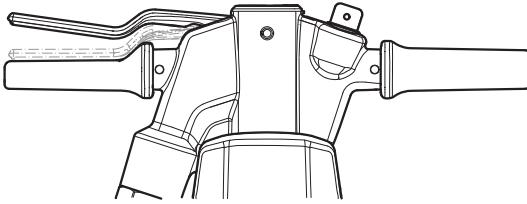
Stop the pneumatic breaker by releasing the start and stop device. The start and stop device will automatically return to the stop position.
